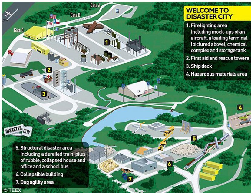
Fig. 11. Schematic showing the layout of Disaster City.
