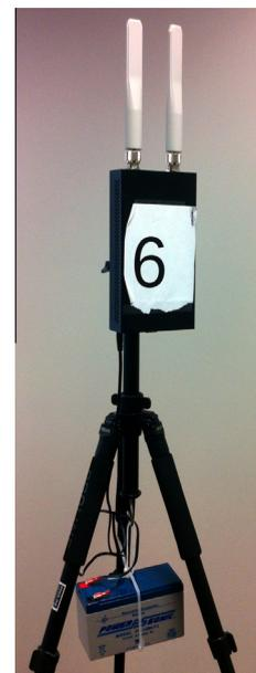
**Fig. 3.** Mikrotik RB433UAH wireless router mounted on a tripod and powered by a battery.
